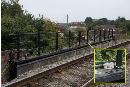
Figure 10. Accelerometers placed on the top flange of the main girder.
