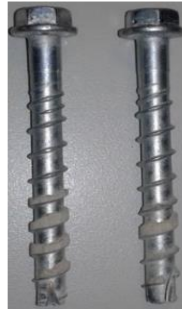
Crushed concrete in between the threads
