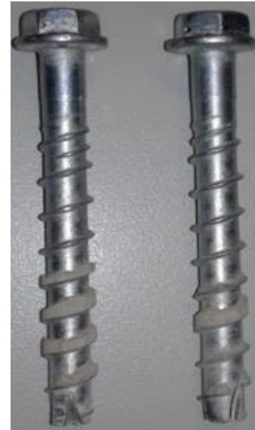
Crushed concrete in between the threads
